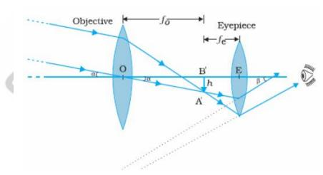
Magnification,  $m = f_o / f_e$  and length of the tube,  $f_o + f_e = L$ 8 =  $f_o / f_e$  and  $f_o + f_e = 36$ Hence, 8 $f_e + f_e = 36$ Or  $f_e = 4$  cm Therefore,  $f_o = 32$  cm b)
