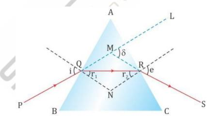
As the ray PQ after refraction from surface AB emerges from face AC at point R of the prism, it implies that the refracted ray QR travels parallel to the base of the prism. This happens at the minimum deviation position.
